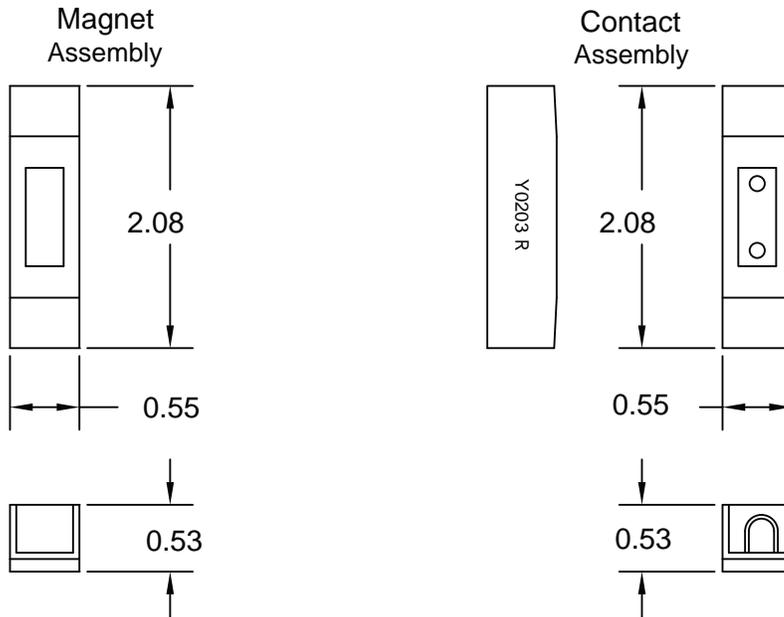
**Installation Features** Screws and wires can be hidden in this contact. Wires can be installed from the top, bottom side or from behind.
