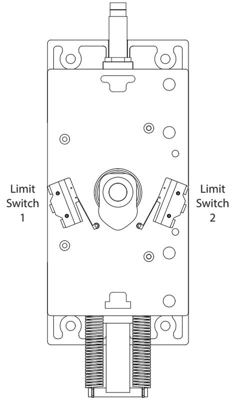
ADA Gate control heads use an oblong lobe shaped limit switch cam. The point of the lobe needs to be facing the index pin (bar with two springs) when the cam is in the home position.
