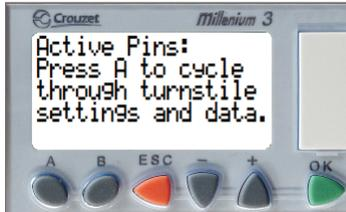
This screen is at the start of the menu cycle. The top section will give a read out of inputs that are currently receiving voltage. The display will return to this screen after cycling through all windows, 5 minutes of inactivity or pressing the B button.
