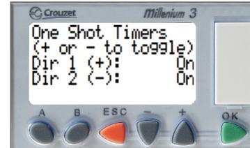
This screen allows for the two one-shot timer settings to be enabled or disabled. This setting prevents access control from holding open a direction on the standard direction inputs. Toggle Direction 1 by pressing + and Direction 2 by pressing -. This should be set to "On" in almost every installation.
