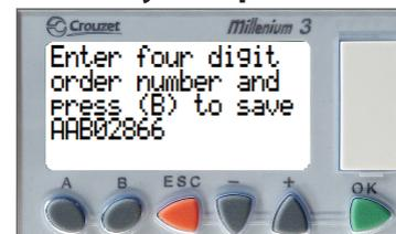
This screen should only appear when first set up in the factory or if something occurs to totally reset the logic controller. If this manages to occur and the order number (if known), enter it as a value then press B to save.
