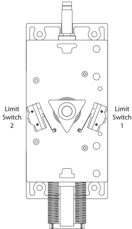
Turnstile control heads use a triangular shaped limit switch cam. One point of the triangle needs to be facing the index pin (bar with two springs) when the cam is in the home position. The two indents in the sides of the triangle are for jiggging purposes. It does not matter which point is facing to the springs.
