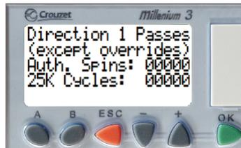
This screen gives statistics about how many times direction 1 was activated and cycled. Since there is a limit to how many counts can be displayed, after 25000 cycles the first counter resets and adds to the second counter.
