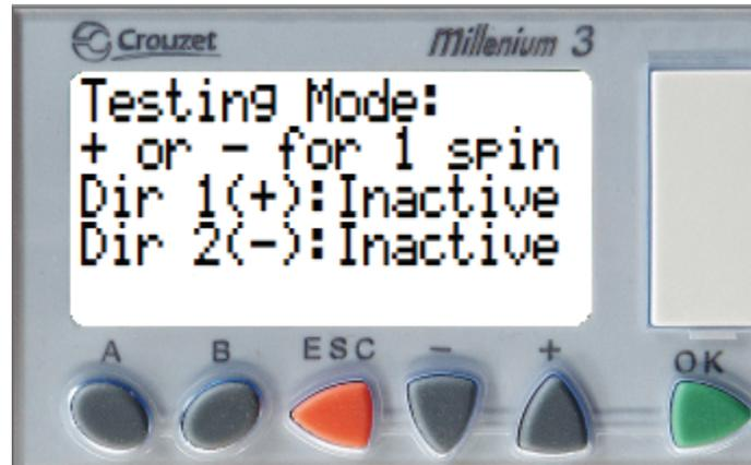
Testing mode simulates valid access control inputs based on the settings defined on the other menu screens. The unit should unlock for the duration of the directional timer or until the unit is rotated. If the button is pressed twice, it should allow two rotations or time out based on the multi-swipe setting. If the button is held and the one shot timers are disabled, the unit will continue to remain open until the button is released and another rotation or timeout occurs.
