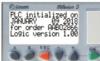
This screen displays when the PLC was initiated, the order number it was activated for (except for any revision suffixes which are not needed for order lookup), and the PLC software version.
