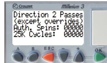
This screen gives statistics about how many times direction 2 was activated and cycled. Since there is a limit to how many counts can be displayed, after 25000 cycles the first counter resets and adds to the second counter.
