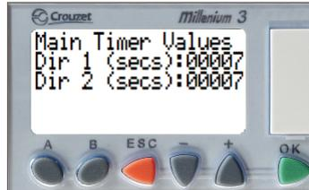
This screen allows for the each directional timer to be modified. Select which value you wish to edit by pressing the + & - key. Press OK to select the value then press + or - to modify. Save by pressing the OK button again. Each timer can have a value of 1 - 60 seconds. The timer will be canceled upon rotation of unit.
