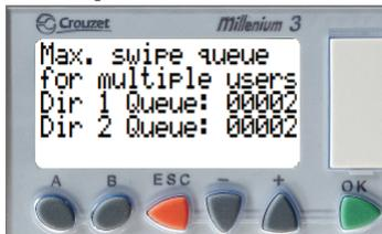
This screen defines the maximum number of access control requests the unit will allow in queue. Each value can be set from between 1 (for maximum security) to 3 (for fast paced passage). The default is 2. The method to change these settings is the same as the Timer Values Screen.
