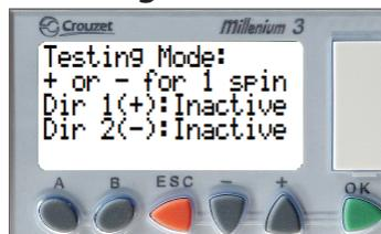
While this screen is active, the unit can be tested with push buttons to simulate access control inputs. See the page dedicated to testing for more information.
