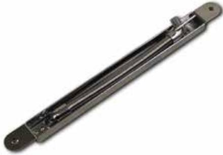
**PT-5** - Power Transfer loops provide a means of running wires from the frame to doors equipped with electric locks and exit devices. The PT-5 is a heavy-duty power transfer device, concealed mortise mount, UL listed miscellaneous fire door accessory. It is UL 10C positive pressure compliant and UBC 7-2 Fire Test for Door Assemblies compliant.
