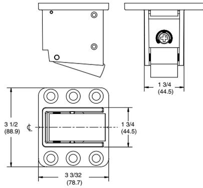
Top fitting has a latch that allows the mullion to be locked back into place without use of the key.
