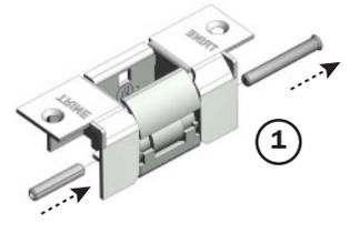
Dimple shows Fail-Safe Slider position
