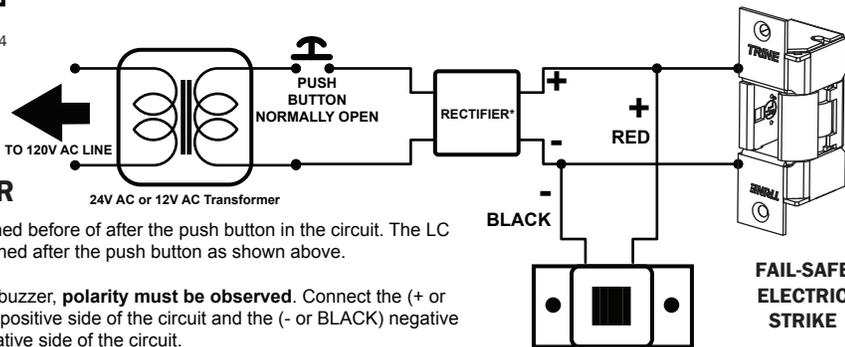
\* The rectifier can be positioned before of after the push button in the circuit. The LC module can ONLY be positioned after the push button as shown above.
