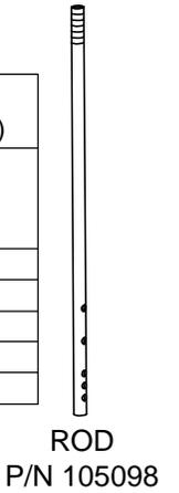
Note: If hole V or W is used (or if new hole is drilled closer to threaded end), trim off UNTHREADED end of rod as needed to allow rod to slide into bottom bolt far enough to pin.
