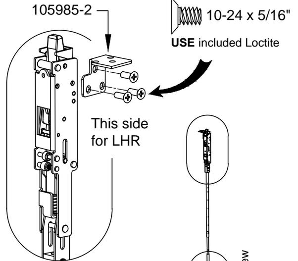
8a THESE 2 SURFACES **MUST** BE ALIGNED WHEN ASSEMBLED AND FACING INNER DOOR FACE
