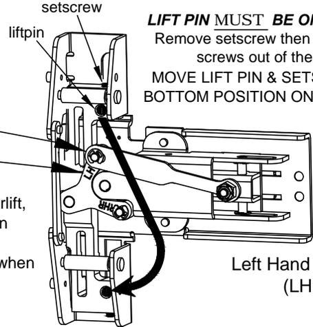
**LIFT PIN MUST BE ON BOTTOM**
