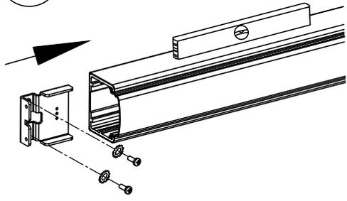
LEVEL device before installing endcap bracket
