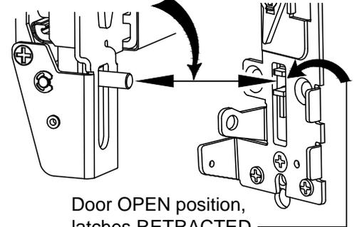
11f CHECKING FOR DEVICE CLEARANCE (Cut-Off procedure if required)
