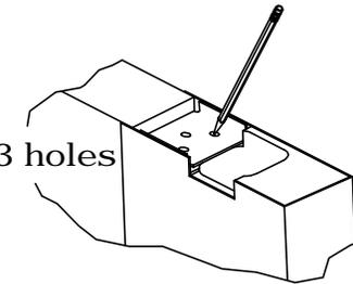
**2c** REMOVE WRAP & DRILL (3) CLEARANCE holes
