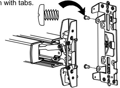
Lift pin protruding from back of centercase **MUST** be inserted **BETWEEN** these two tabs.
