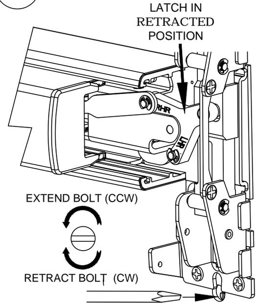
13e: **BOTTOM LATCH ADJUSTMENT:** With pushpad depressed (retracted position), extend or retract bottom bolt to desired engagement and clearance.
