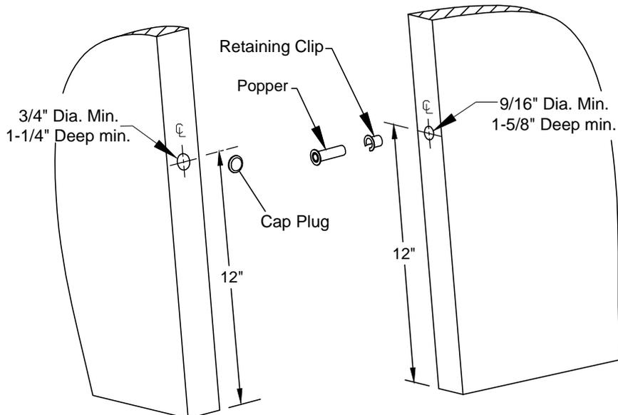
**NOTE:** Door/Frame reinforcement is required where popper and cap plug are to be installed.
