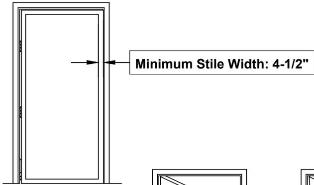
Doors and frames with walls having a structural thickness (metal skin plus reinforcement) to engage less than (3) full screw threads, are considered unreinforced for hardware.
