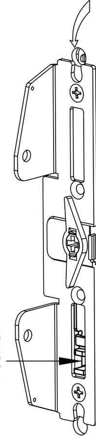
With latch bolt extended, top adjustment screw should be exposed.
