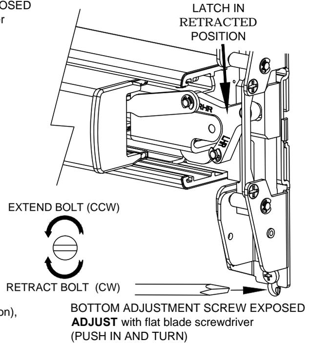
13e: **BOTTOM LATCH ADJUSTMENT:** With pushpad depressed (retracted position), extend or retract bottom bolt to desired engagement and clearance.
