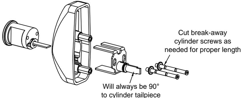
**6. GO BACK AND FOLLOW EXIT DEVICE INSTRUCTION STEPS** up to, but not including ASSEMBLE DEVICE TO DOOR. Trim must be installed **BEFORE** device is assembled to door.
