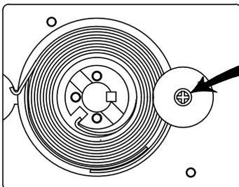
Remove the 10-32 screw and two Round Stops.
