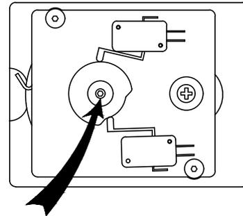
Mark Cam position. If no parts are broken this will aid in the reassembly process.
