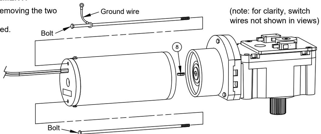
Examine motor shaft for excessive wear in key slot. Replace motor if necessary.
