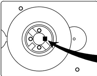
To replace the shaft, turn unit upside down. Tap the top on a hard surface or carefully tap the SPLINED end of the shaft with a flat face hammer until the key from the Arbor and the Shaft can be removed. If this fails, drill with 1/8" drill bit, insert an easy-out (a small screw may work) and pull key out.
