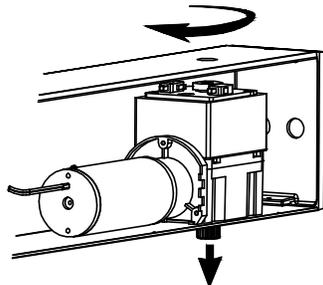
Rotate ASSEMBLY into enclosure, letting shoulder of gearbox drop down into shaft hole. Align screw holes at bottom and apply **blue thread locker** to all 4 screws before tightening
