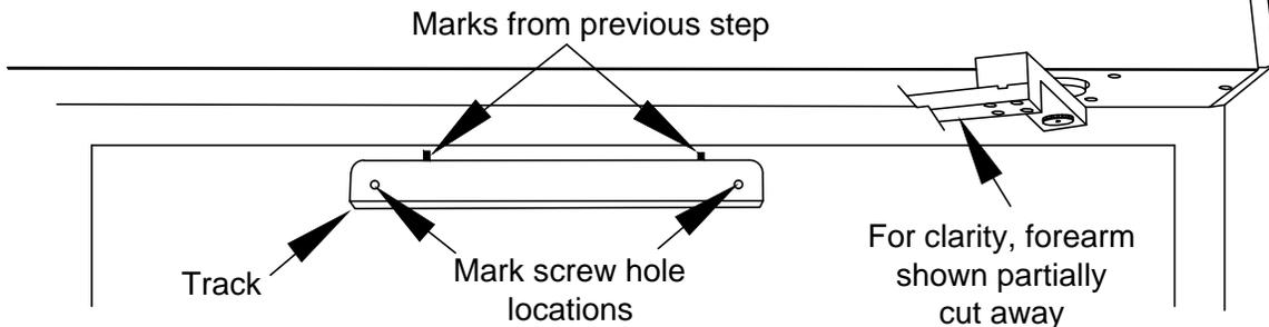
Using the screws & lockwashers provided, install the track with the slide block in place on the arm pin.
