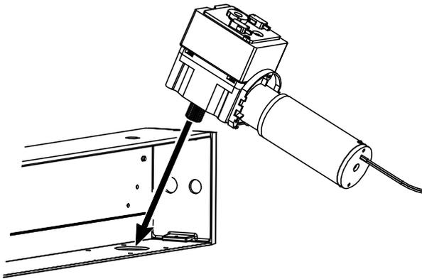
With ASSEMBLY perpendicular to enclosure, insert splined shaft into shaft hole
