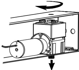
Rotate ASSEMBLY into enclosure, letting shoulder of gearbox drop down into shaft hole. Align screw holes at bottom and apply **blue thread locker** to all 4 screws before tightening
