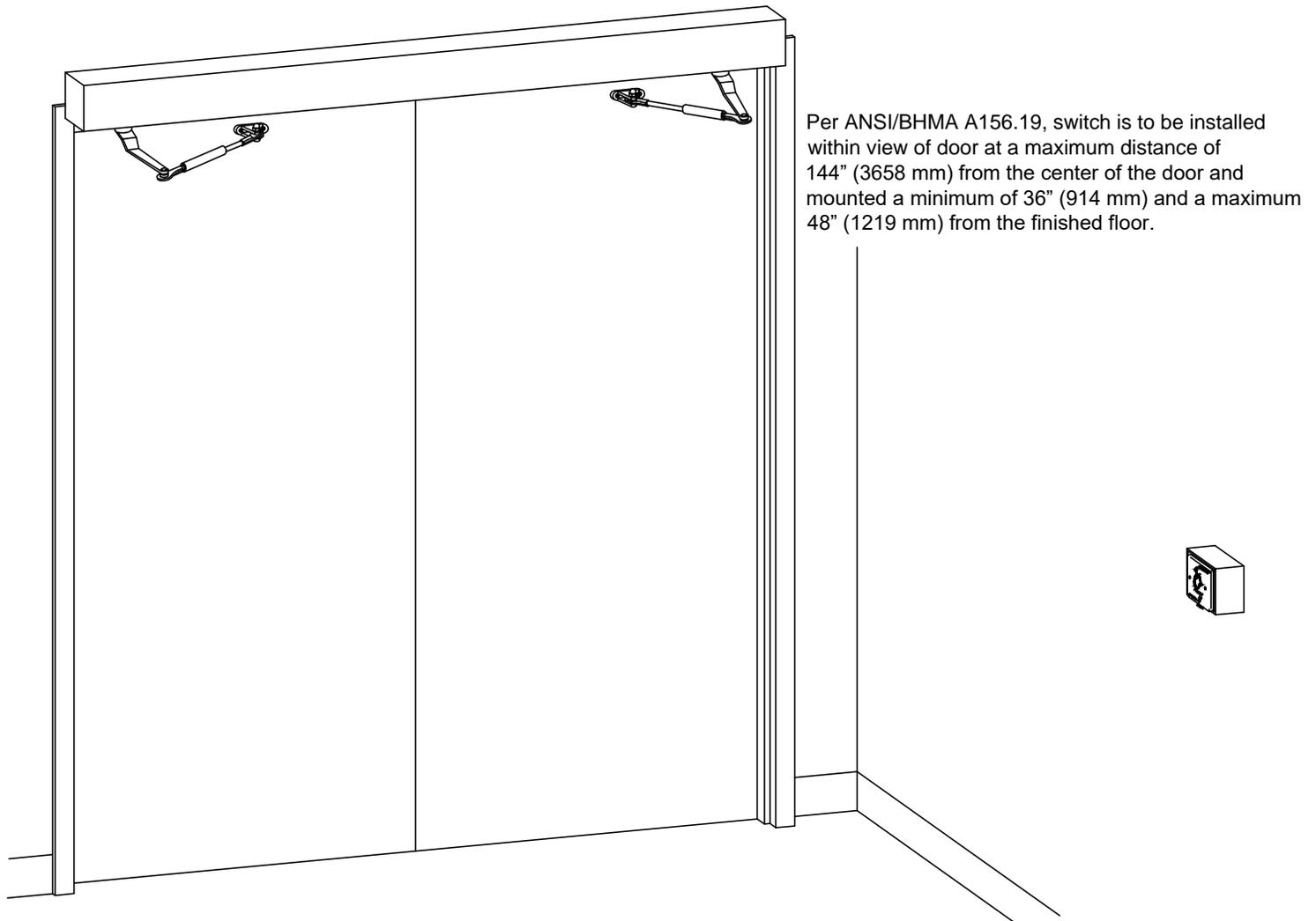
Per ANSI/BHMA A156.19, switch is to be installed within view of door at a maximum distance of 144" (3658 mm) from the center of the door and mounted a minimum of 36" (914 mm) and a maximum 48" (1219 mm) from the finished floor.
