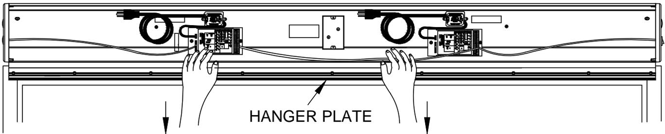
Lift the operator and lower onto the webs of the hanger plate bracket. Be sure both top and bottom are engaged.
