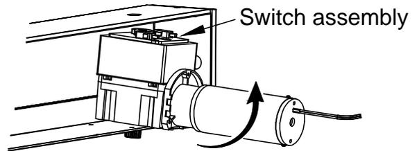
Rotate ASSEMBLY to an almost horizontal position being careful not to let switch assembly hit enclosure
