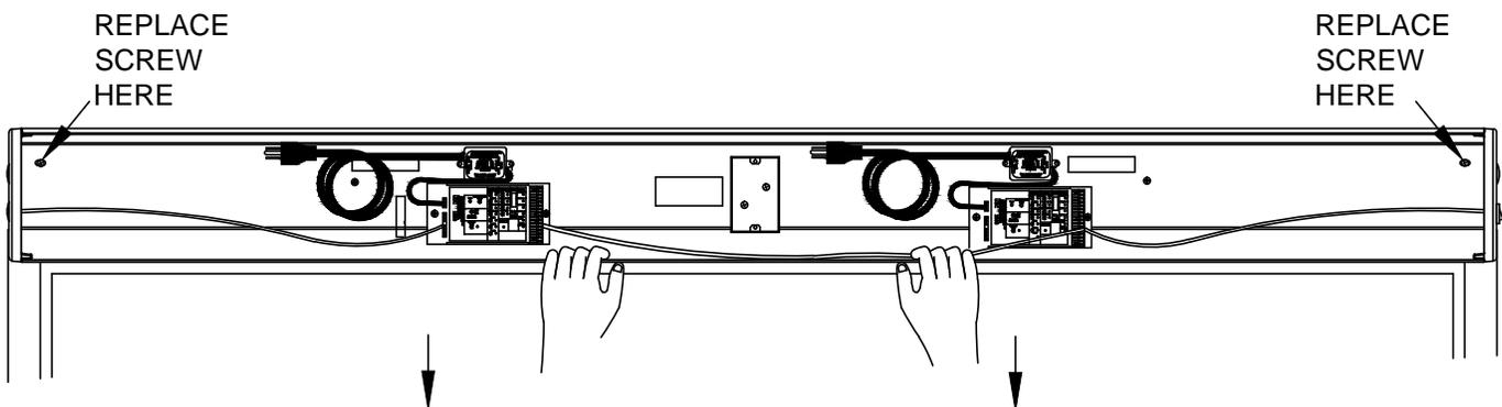
Once they are seated, pull down until unit is completely flush and screws can be replaced in top corners.
