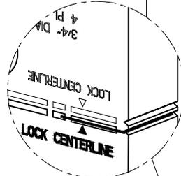
Align the plastic template LOCK CENTERLINE with the mark previously made as shown. Mark the four A locations.
