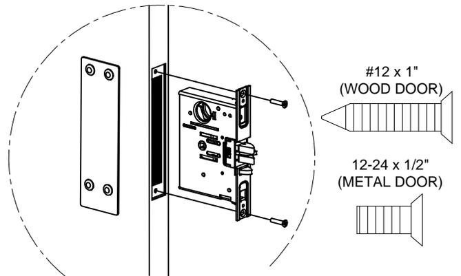
Note: Mortise lock and mounting hardware supplied with exit device. Fasten screws loosely.
