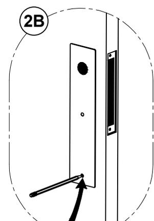
Mark and drill 3/8" diameter (1/2" max) hole thru door
