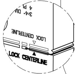
Align the plastic template **LOCK CENTERLINE** with the mark previously made as shown. Mark the four **A** locations and the **03 INPUT** location.
