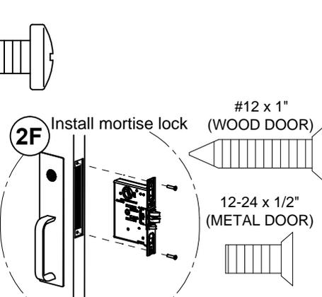
Mortise lock and mounting hardware provided with exit device. Fasten screws loosely.
