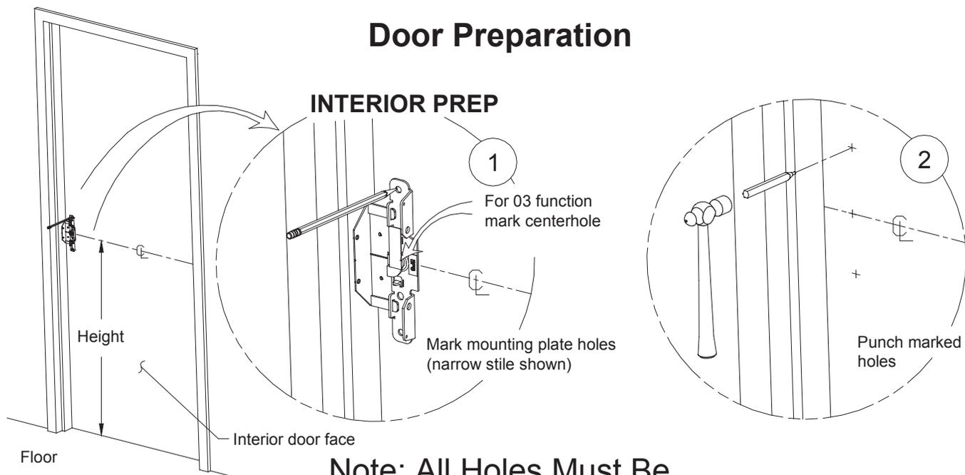
**Note: All Holes Must Be Drilled Straight and Level**
