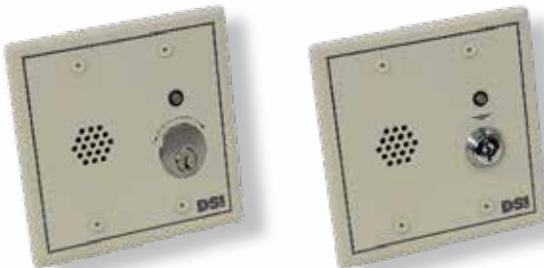
The ES4300A series, used as a stand-alone device or tied to any access control system, provides security for emergency exits. This device activates a local audible alarm and a remote alarm contact when an exit violation occurs. Once triggered, the ES4300 remains in alarm until reset by the auto reset feature, the integral key switch or remotely through a dry contact. The ES4300A is now available with an optional tamper switch.
